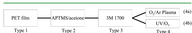
Figure 2. Various processes to pattern PET surfaces into different regions with controlled wettability.
